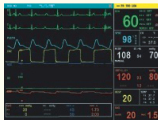
Multi-Gas Measuring To measure the concentration of EtCO 2 , N 2 O, O 2 and other five anesthesia gases, including Des, Enf, Sev, Hal, Iso
