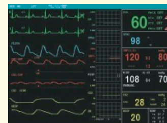
"Trend Screen" Mode To display the trend data along with the waveforms and measured values (Trend time length: 2 hours)
